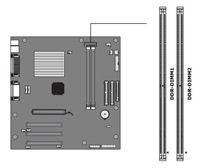
Both sides of each Double-data rate, Dual Inline Memory Module (DDR-DIMM) look very similar. The side with pin 1 has a small "1" to the left of pin 1. Be sure to orient the memory module correctly in the DDR-DIMM slot (a small triangle on the slot indicates pin 1).
